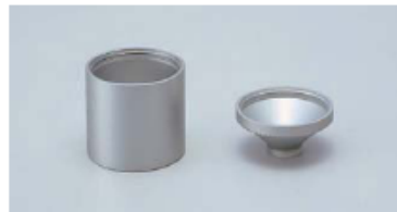
Glass Light-Projection Tube CR-A33f (For CR-400) and CR-A33e (For CR-410) Glass Light-Projection Tube CR-A33f and CR-A33e have a glass plate at the tip and can be used for measuring wet surfaces or for ensuring that materials such as textiles are flat during measurements.
